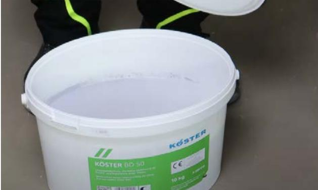
KÖSTER BD 50 must be stirred for a minute in the original bucket to reach a homogenous consistency before using.
